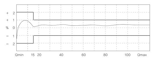
$\pm 1.5\%$  for Qmin to 0.15 Qmax  $\pm 1$  for 0.15 Qmax to Qmax
